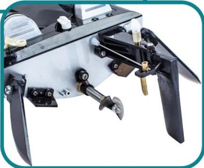
With water-cooling system motor and ESC, excellent cooling down performance, which make the boat more stable in a longer time racing.
