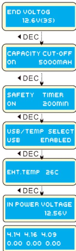
The first screen (End Voltage) shows the voltage terminal, which will be achieved when the charging process completes.
